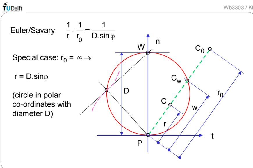
Fig. 4.4.2 Inflection circle: locus of points of the moving plane with  $r_0 = \infty$
