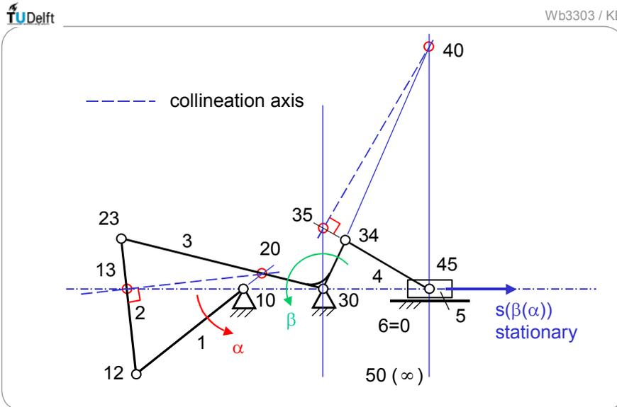
Fig. 4.3.2 Stationary motion with series connection (simultaneous extreme values of 1st order transfer function)
