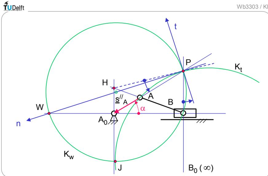
Fig. 4.7.2 Construction of the 2nd order pole J directly with Bresse's circles (slider-crank mechanism)
