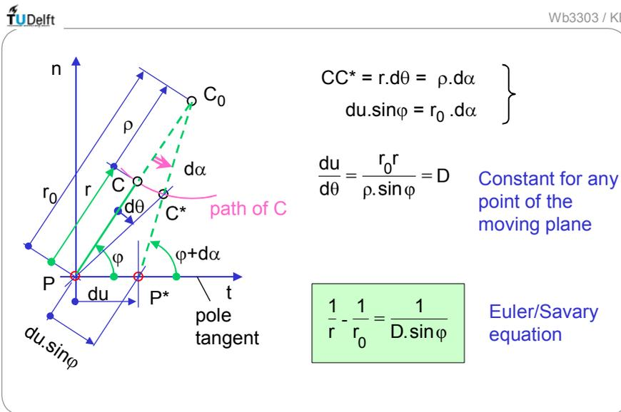
Fig. 4.4.1 Radius of curvature  $\rho = r_0 - r$  acc. Euler/Savary
