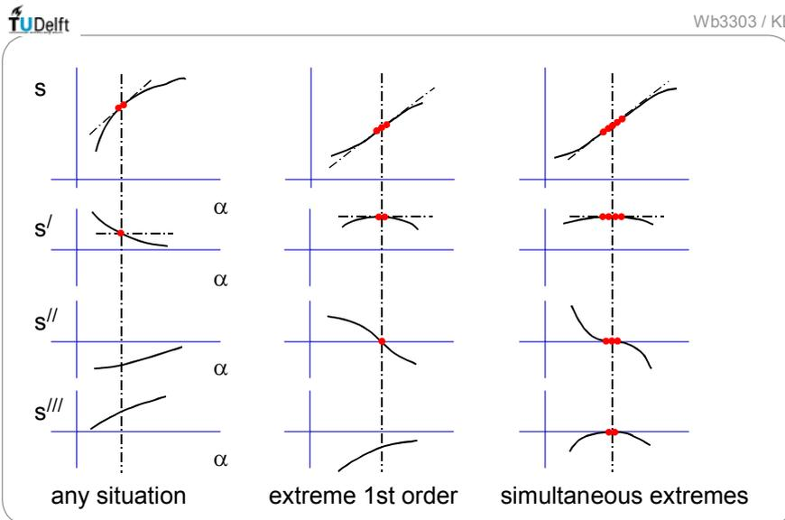
Fig. 4.3.3 Quality of stationary motion, with number of points coinciding with ideal line
