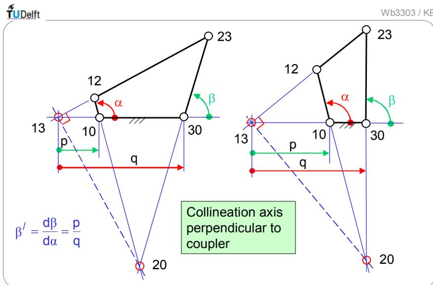
Fig. 4.3.1 Extreme values of first order transfer function  $d\beta/d\alpha$  (acc. Freudenstein/ Meyer zur Capellen)
