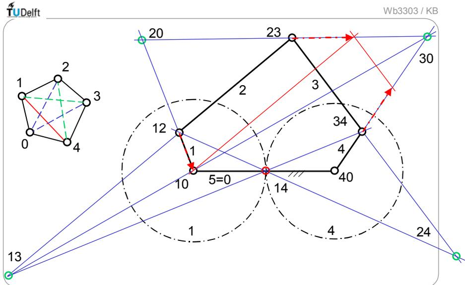
Fig. 4.2.2 Construction of first order poles and motion vectors of a geared five-bar linkage (acc. Aronhold/Kennedy)
