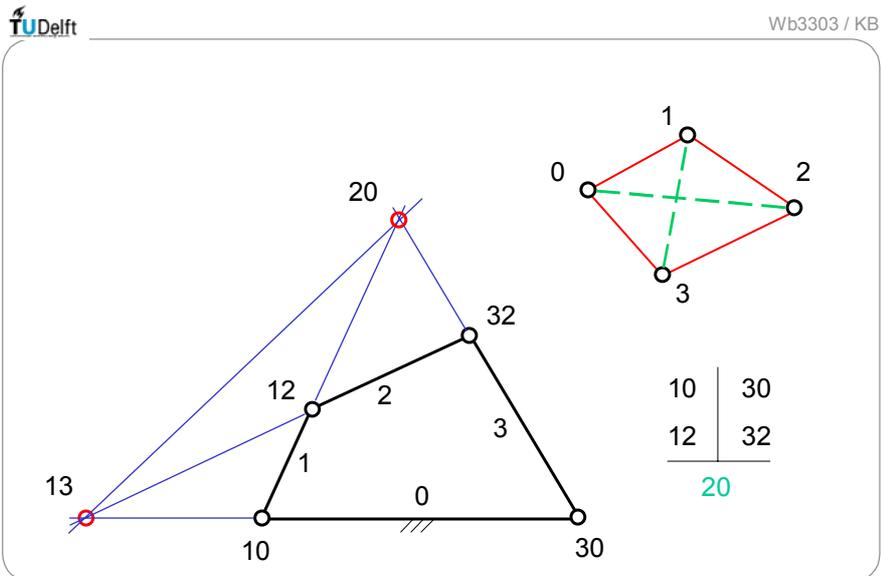
Fig. 4.2.1 Dual configuration of relative poles (acc. Aronhold/Kennedy)
