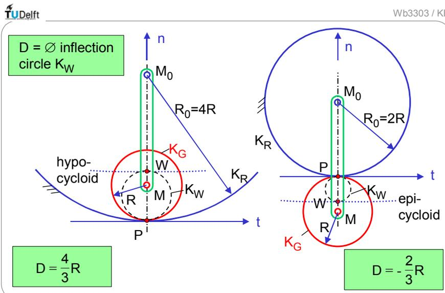
Fig. 4.6.1 Cycloids approximating a straight line
