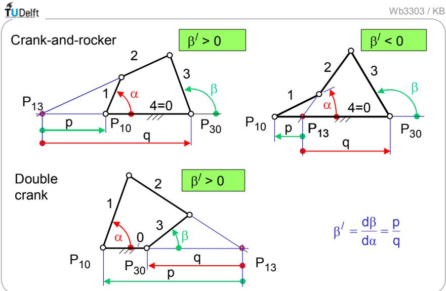
Fig. 4.1.3 First order transfer functions and pole distances  $p$  and  $q$
