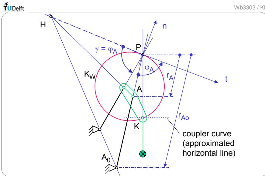
Fig. 4.6.2 The inflection circle used in crane design
