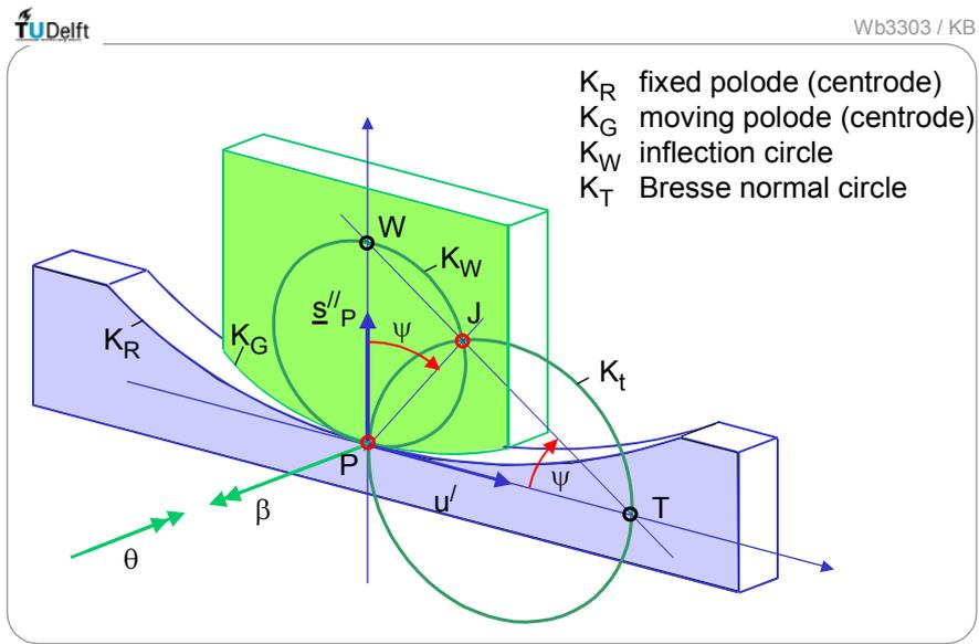
Fig. 4.7.1 *Inflection circle and Bresse Normal circle of a moving plane*
