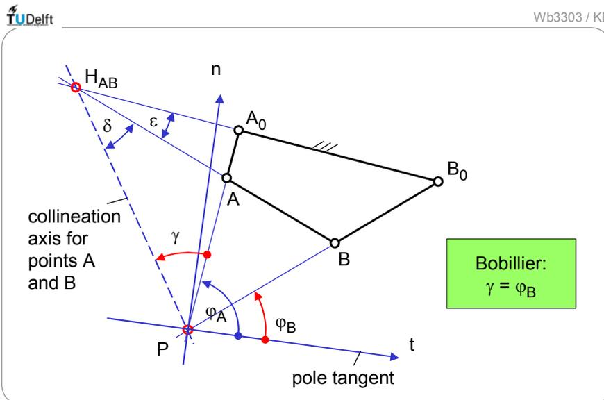
Fig. 4.5.1 Method of Bobillier/Aronhold for construction of the pole tangent
