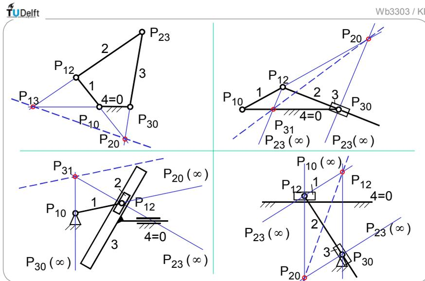
Fig. 4.1.2 First order poles of the Four-bar linkage.
