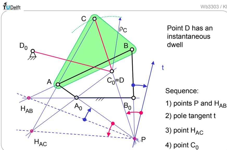
Fig. 4.6.3 Construction of radius of curvature using Bobillier/Aronhold twice (6-bar dwell mechanism)
