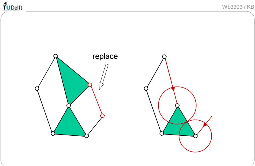
Fig. 2.7.6 Replacement of a binary link in a four-bar chain by a pair of gears (example with chain of Watt)
