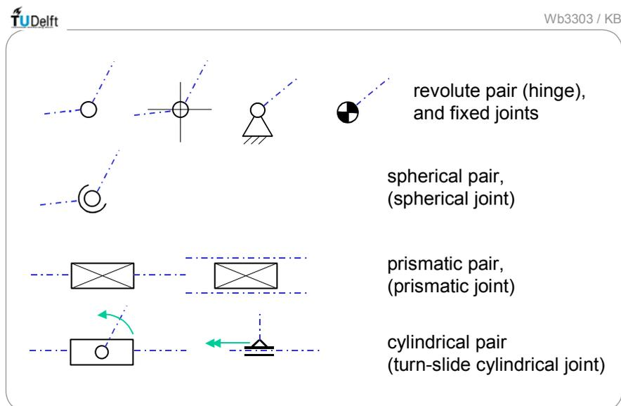
Fig. 2.1.3 Typical graphical representation of joints
