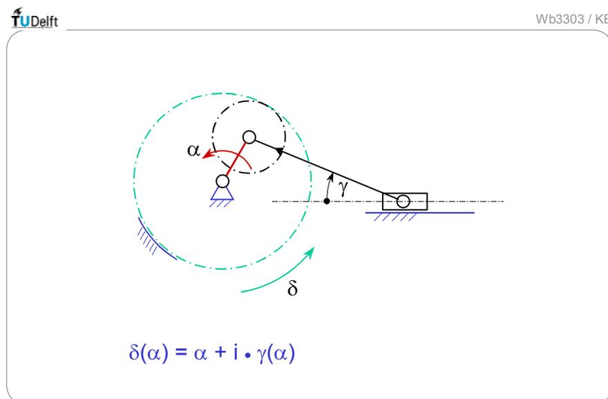
Fig. 2.7.7 Superposition of transfer functions in the Watt-chain: the basis idea for step-dwell-step motion
