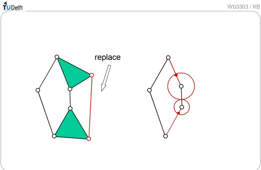
Fig. 2.7.8 Replacement of a binary link in a four-bar chain by a pair of gears (example with chain of Stephenson)
