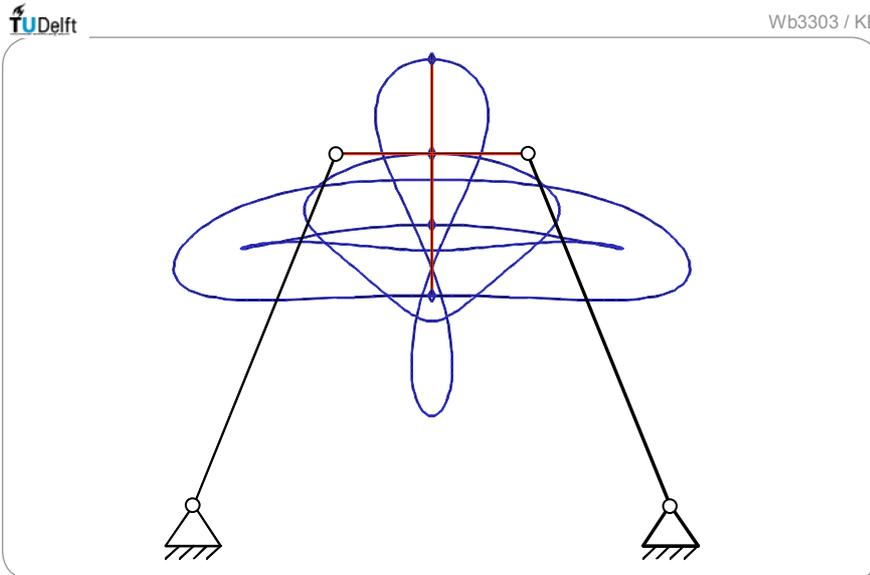
Fig. 2.4.3 Examples of coupler curves generated by a four-bar linkage (symmetrical curves)
