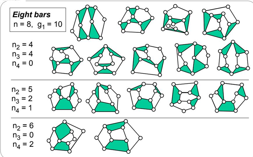
Fig. 2.3.2 Basic kinematic chains with 8 bars and  $F=1$
