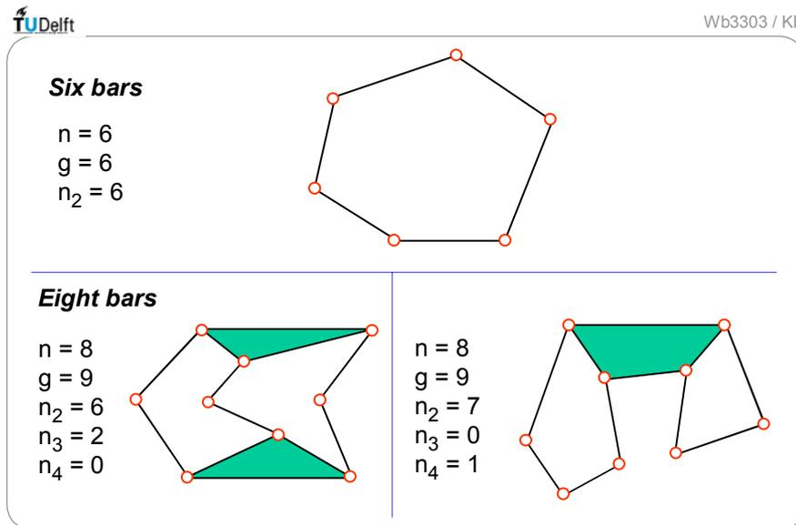
Fig. 2.6.4 Closed chains with  $F=3$
