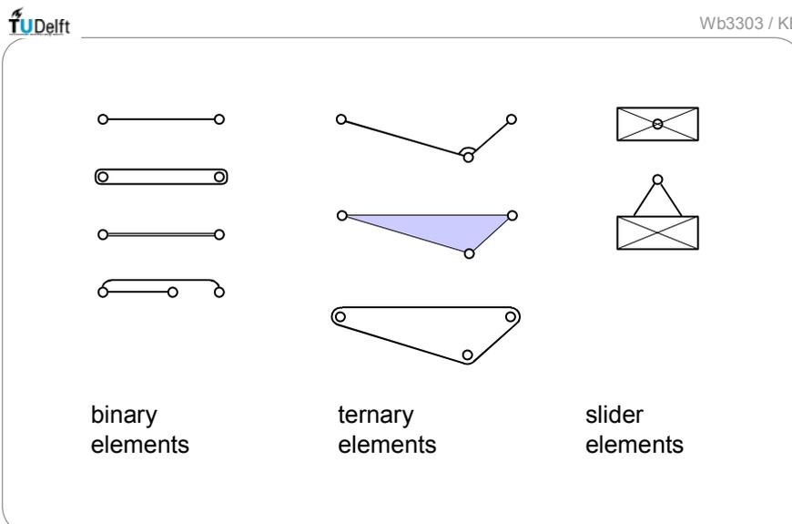
Fig. 2.1.2 Typical graphical representations of elements
