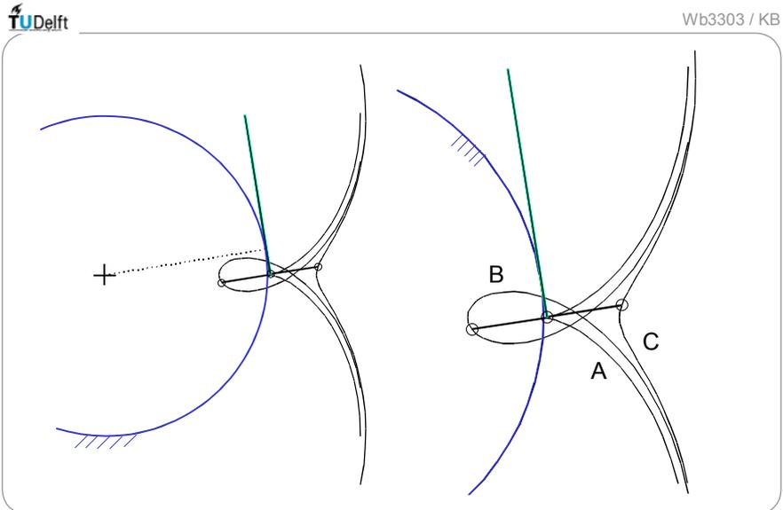
Fig. 2.7.5 Circle-involutes, pointed (A), waved (B) and curled (C)
