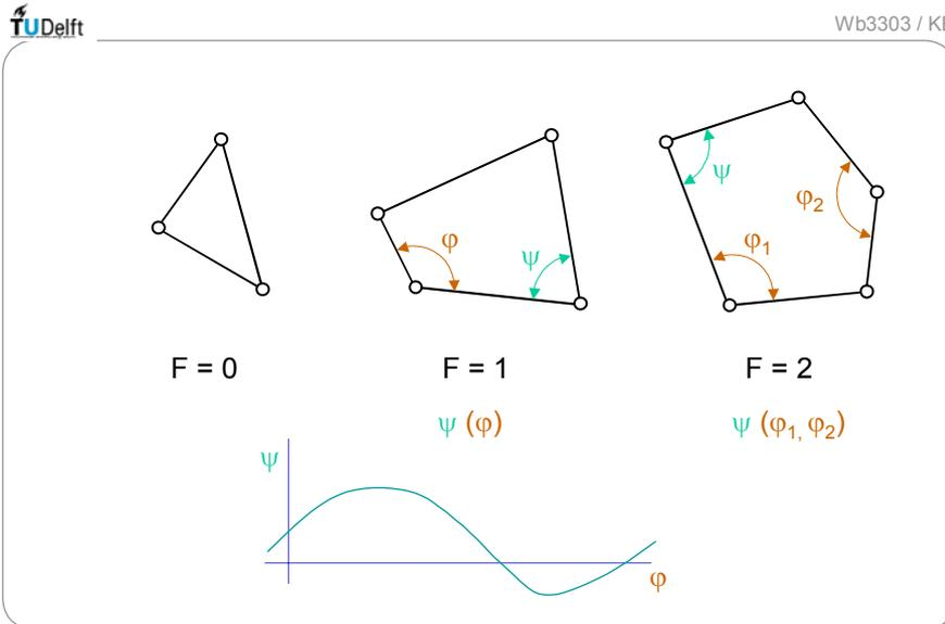
Fig. 2.2.1 Mechanisms and Degree of Freedom  $F$  (mobility)
