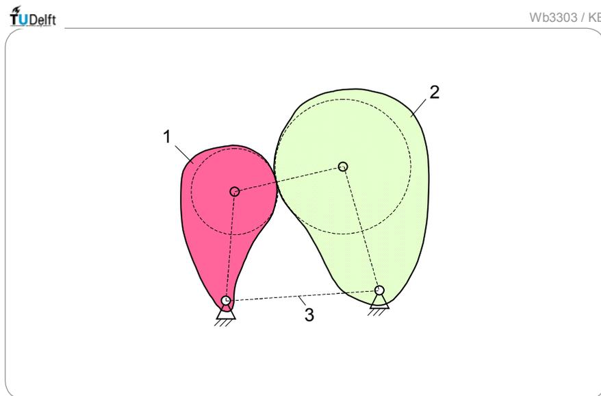
Fig. 2.8.1 Instantaneous equivalence of three binary links and two curves with sliding and rolling contact
