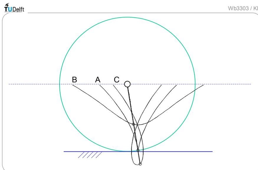
Fig. 2.7.4 Ortho-cycloids, pointed (A), waved (B) and curled (C)
