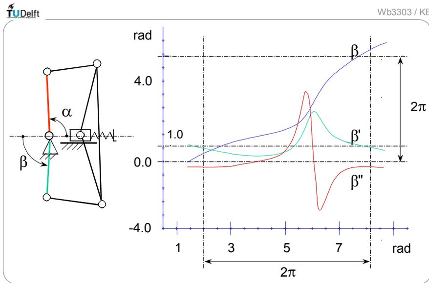
Fig. 2.5.2 Watt-2 mechanism used as a series connection of two double crank mechanisms (adjustable frame link).
