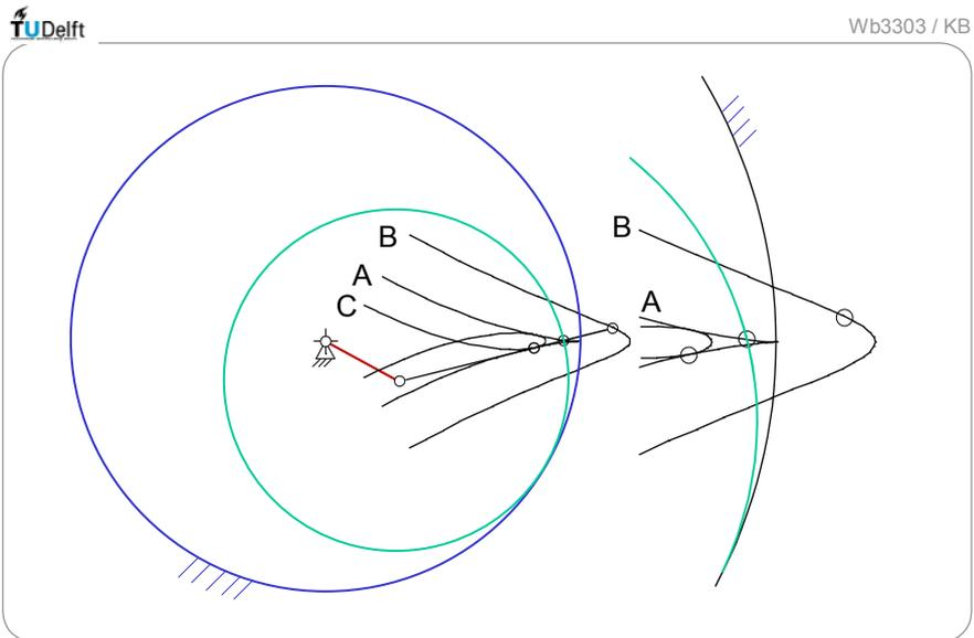
Fig. 2.7.3 Hypo-cycloids, pointed (A), waved (B) and curled (C)
