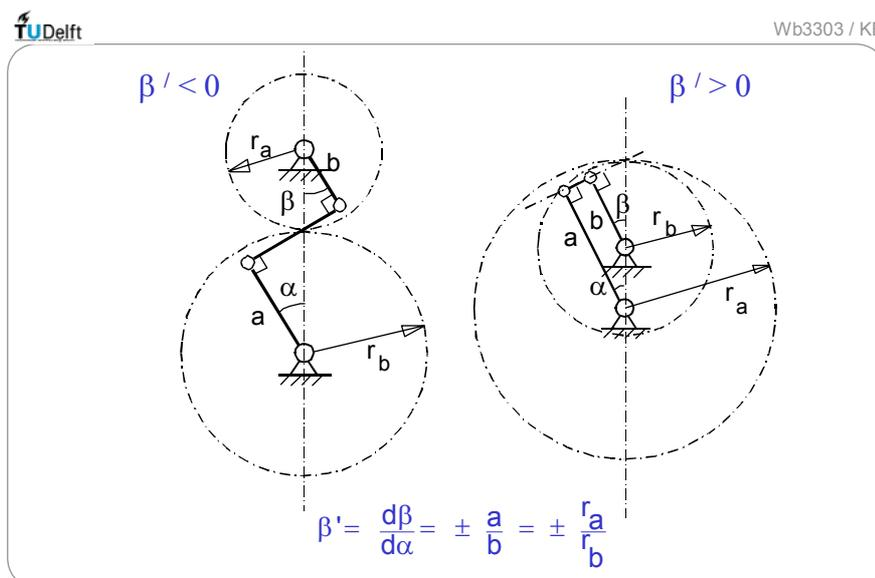
Fig. 2.7.1 Instantaneous equivalence of a gear pair and a four-bar linkage
