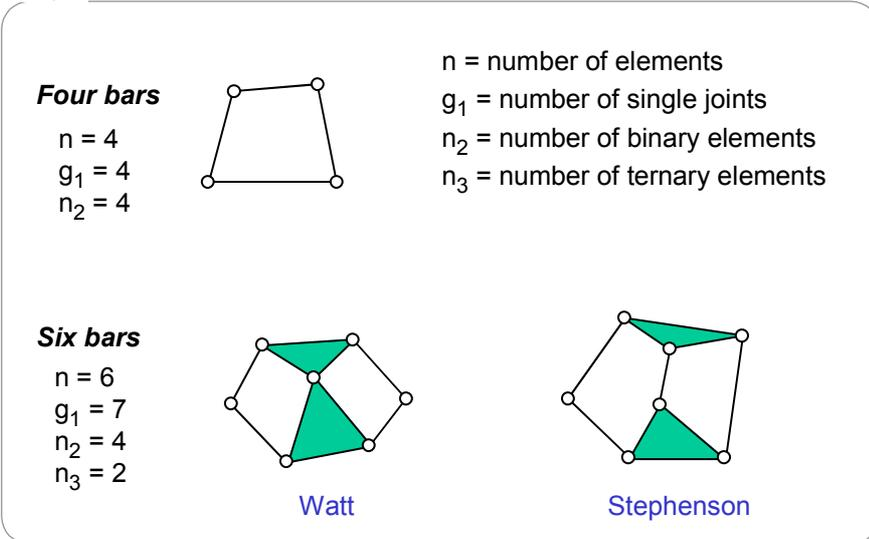
Fig. 2.3.1 Basic kinematic chains with 4 and 6 bars
