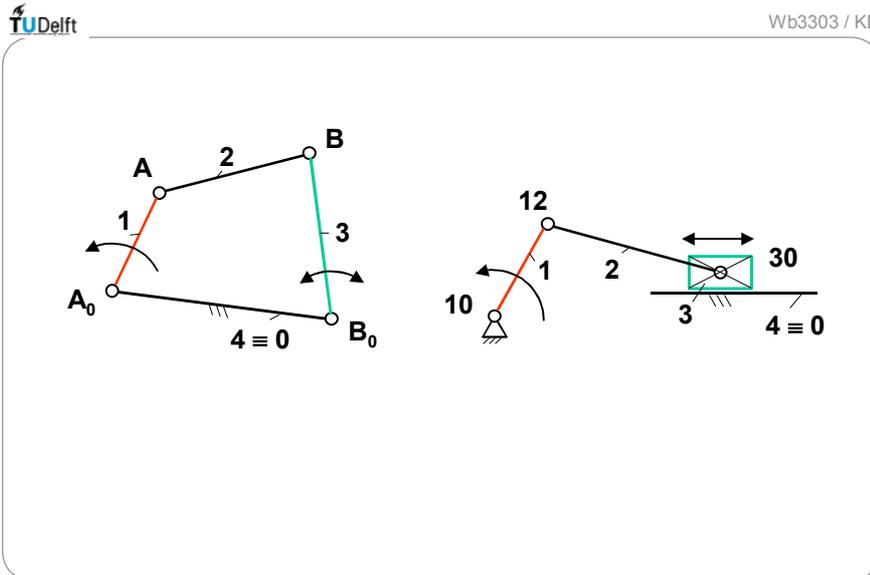
Fig. 2.1.1 Typical graphical representation of mechanisms, with indication of links, joints and input - output
