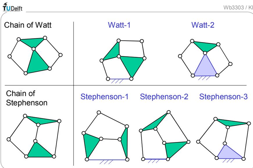
Fig. 2.5.1 Different six-bar mechanisms by fixed link choice
