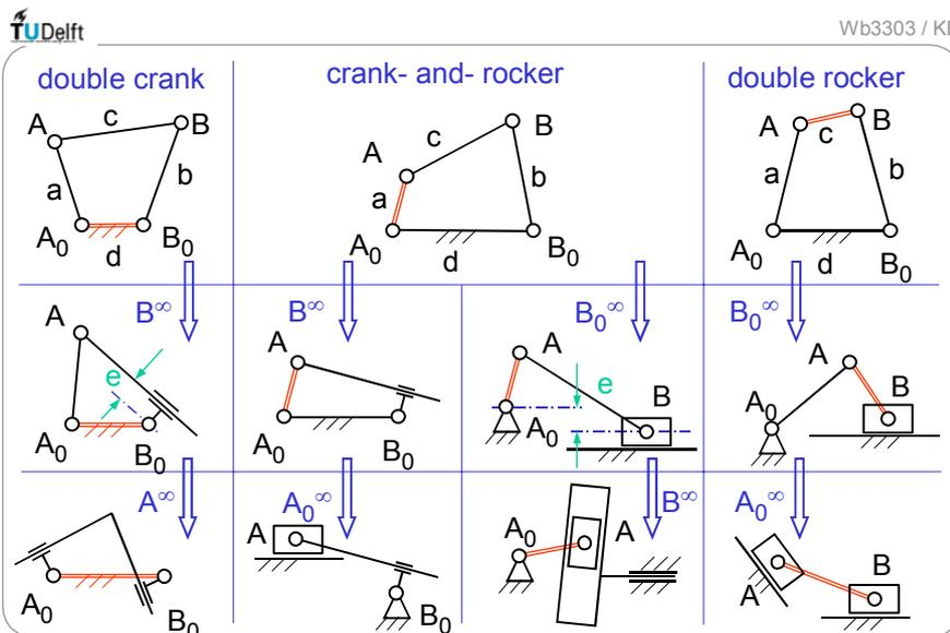
Fig. 2.4.2 Different mechanisms with respect to motion type
