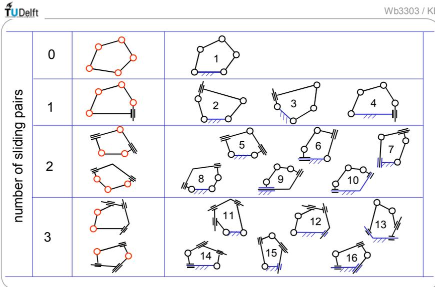
Fig. 2.6.2 Kinematic configurations with  $F=2$  based on the closed chain with 5 bars
