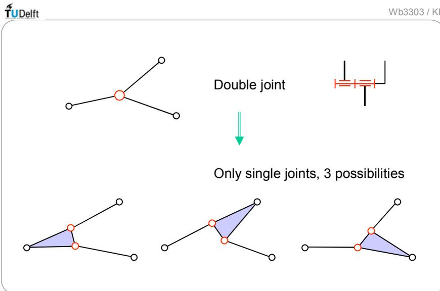
Fig. 2.2.2 Double joint replacement:
