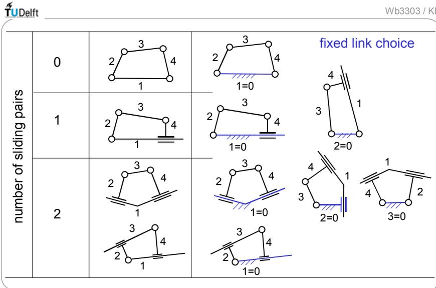
Fig. 2.4.1 Kinematic configurations based on the four-bar chain, revolute pair → sliding pair replacement
