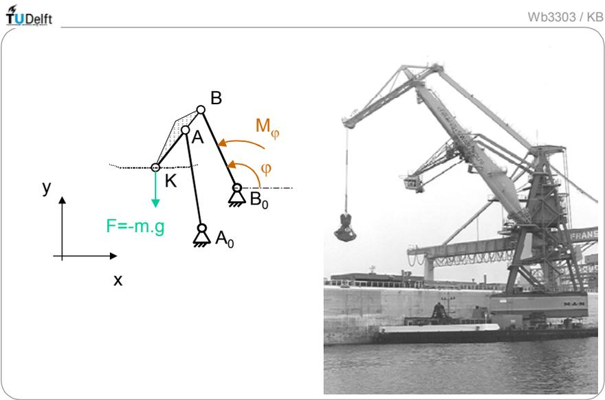
Fig. 1.2.1 Harbour crane (level luffing crane)
