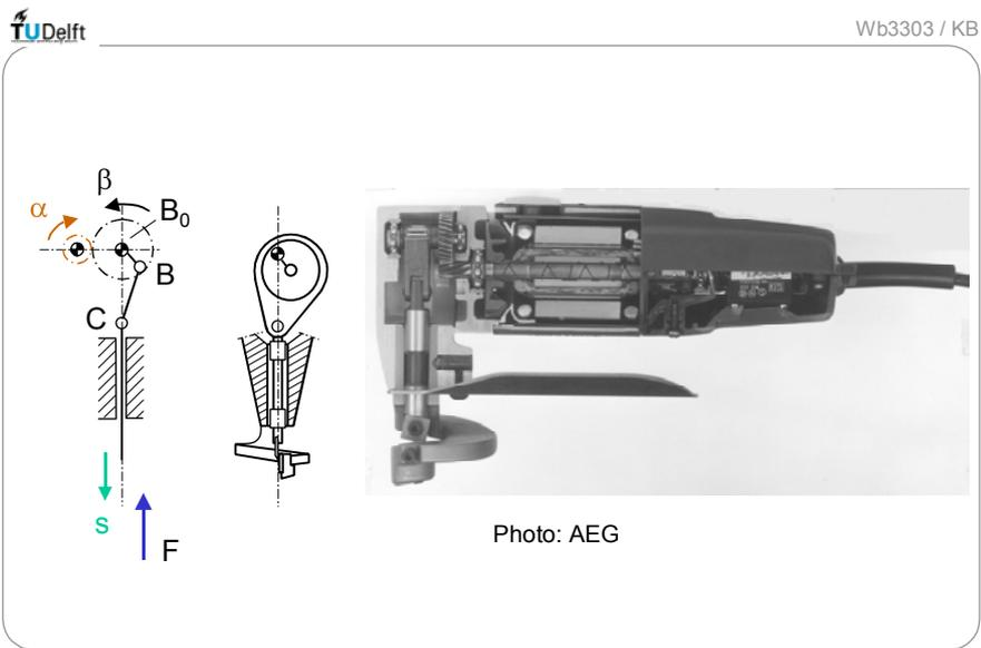
Fig. 1.2.2 Cutting device
