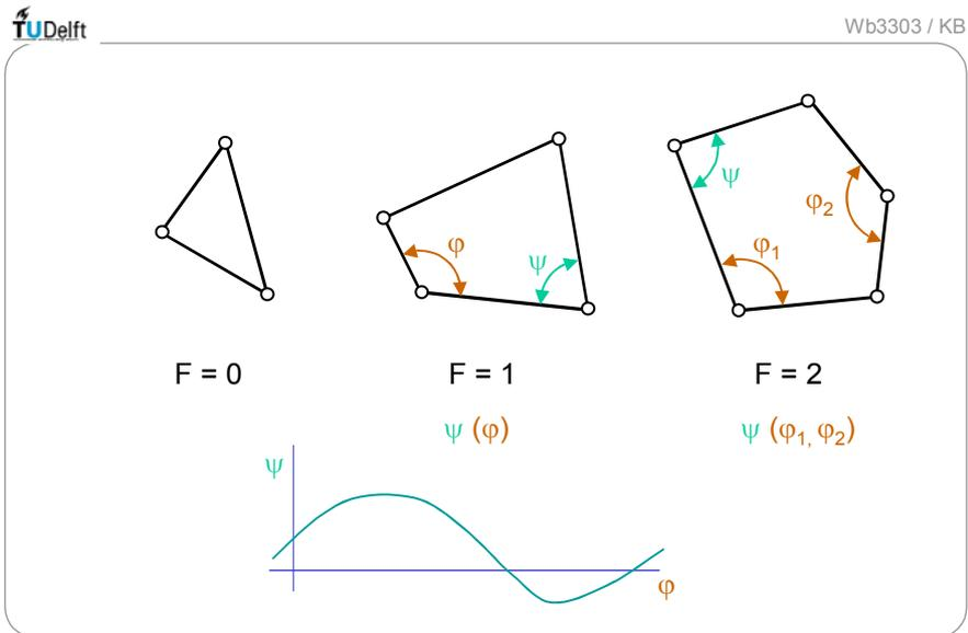
Fig. 1.1.1 Mechanisms and Degree of Freedom  $F$  (mobility)
