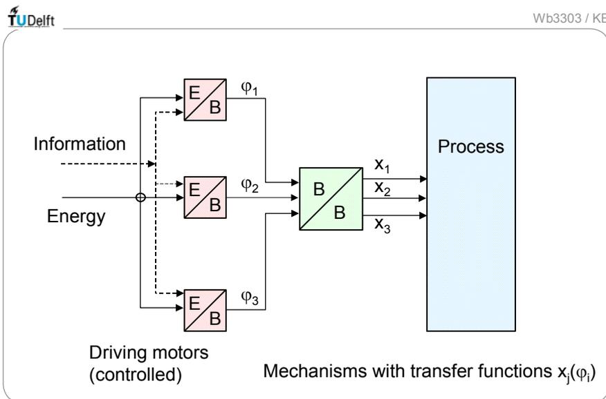
Fig. 1.5.3 Machine concept with multi-degree of freedom mechanism (industrial robot)
