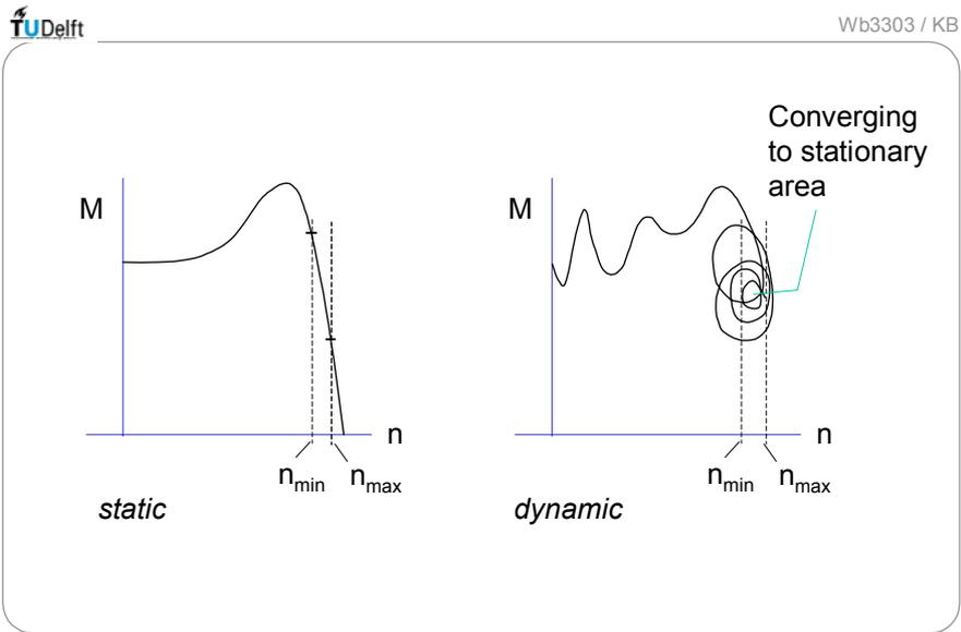
Fig. 1.4.1 Static drive characteristic and typical dynamic behaviour with a mechanism
