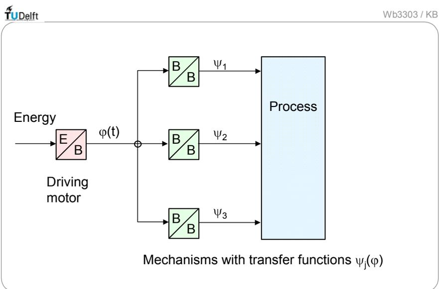
Fig.1.5.1 Machine concept with central driving shaft
