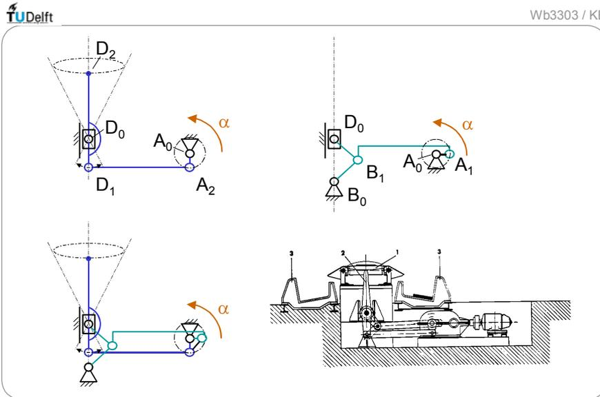
Fig. 1.2.5 Strip stacker mechanism, kinematic scheme
