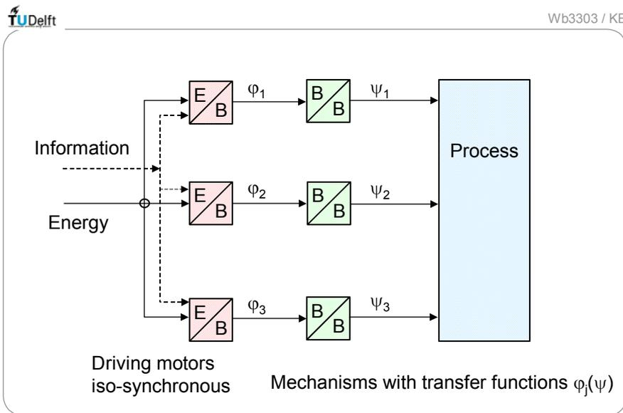
Fig. 1.5.2 Machine concept with distributed driving shafts
